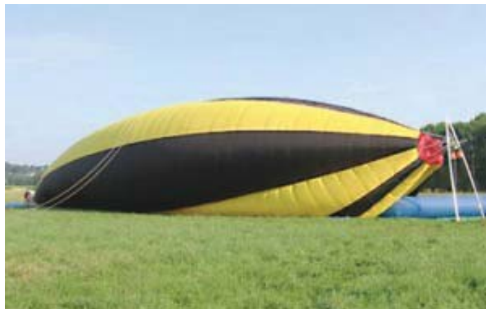
A duct (blue-colored tube) that carries air from the fan into the bottom of the ship is visible on the right side of the photograph. The envelope is filled about half-way with cold air before the burners are fired up.
