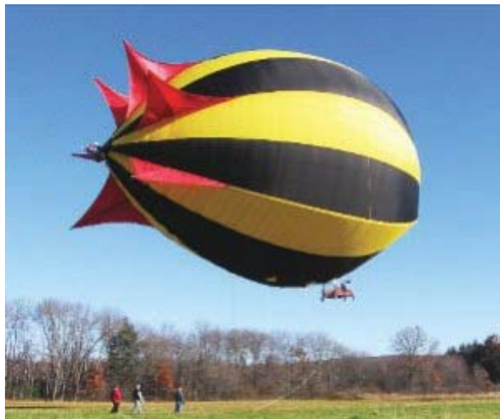
The 205,000-cu-ft hot-air blimp with a ribbed envelope flies for the first time.
